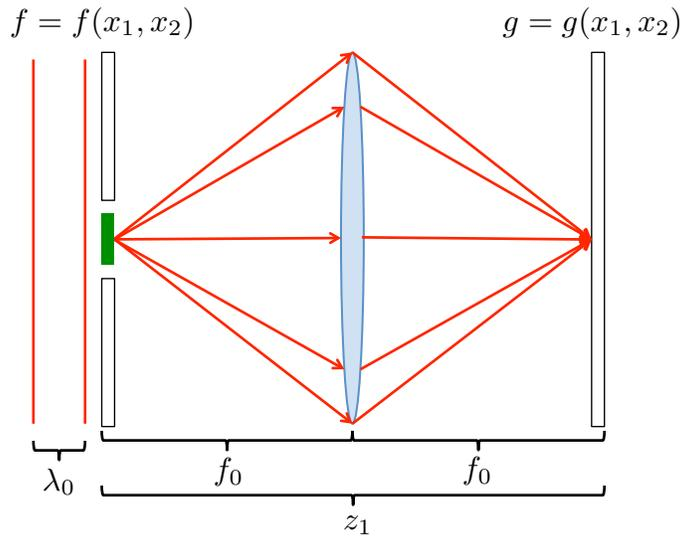
(b) Modified setup with a lens. Here  $f_0$  denotes the focal distance of the lens.
